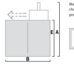
Machine weight total: 522 kg chamber only: 365 kg press unit only: 157 kg
